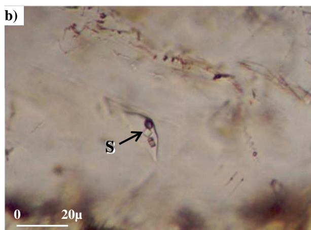
Figure 2. Transmitted light photomicrographs of primary (LV-LV h ) type inclusions, hosted by tourmaline, containing chloride solid phase. (a) sample FM207a (b) sample FM207b.
